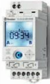
Type 12.A2.8.230.0000 2 CO (DPDT) 16 A 110...230 V AC/DC Enr. 14 002 15
